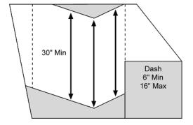
In the above example, the top trailing edge of the dash defines the vertical plane that is used to establish the front-to-back Free Space area. This example also depicts how changes to the roof build-down and floor build-up can be made provided a minimum al distance of 30 inches is maintained. Not to Scale.
