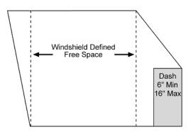
In the above example, the OEM top windshield frame defines the vertical plane that is used to establish the front-to-back Free Space area. (Note how the dash is located completely beneath the OEM windshield location.) Not to Scale.
